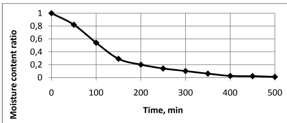
**Fig. 2.** The drying kinetics for mint leaves at  $T=36\text{ }^{\circ}\text{C}$ ,  $RH=40\%$  and  $u=0,22\text{ m/s}$
