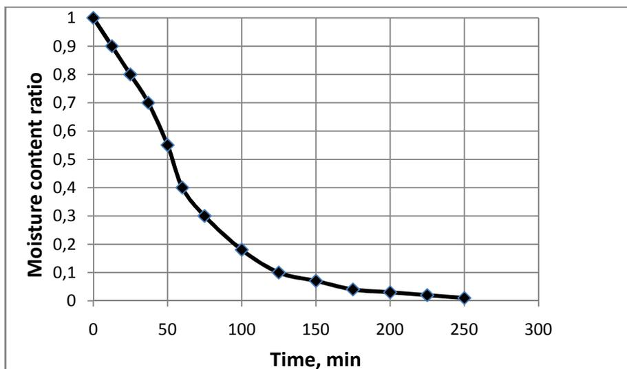
**Fig. 1.** The drying kinetics for nettle leaves at  $T=36\text{ }^{\circ}\text{C}$ ,  $RH=40\%$  and  $u=0,22\text{ m/s}$
