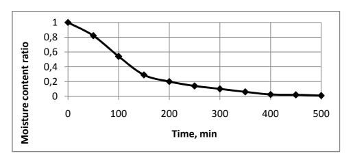
Fig. 2. The drying kinetics for mint leaves at T=36 °C, RH=40 % and u=0,22 m/s
