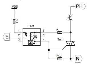
Fig. 3. Schematic realization of the power switch
