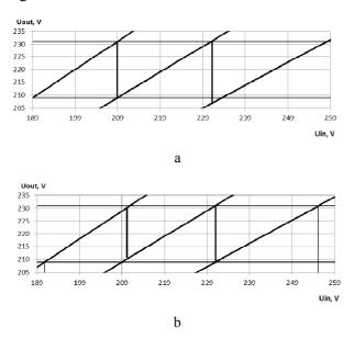
Fig. 2. Dependences of the output voltage on the input voltage with different transformation coefficients: (a) – for  $k_{tr1} = 9.5$ ; (b) – for  $k_{tr2} = 10.5$ )
