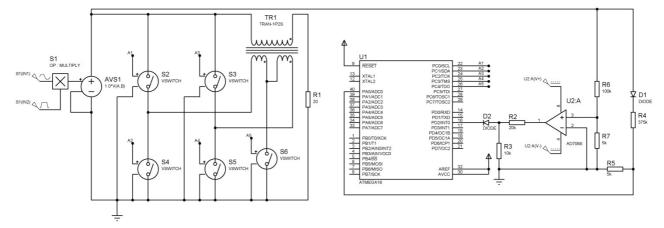
Fig. 4. Virtual model of discrete voltage stabilizer with control system
