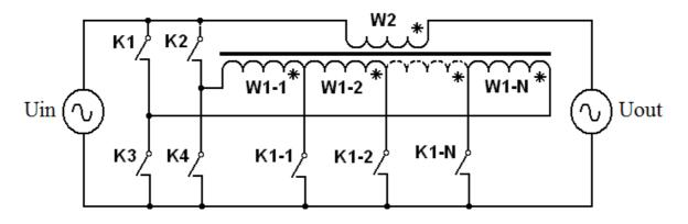
Fig. 1. Structure of the discrete voltage stabilizer
